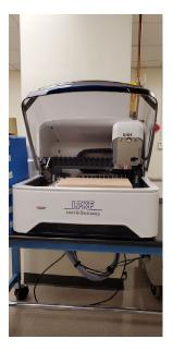
For safety purposes the machine will not move while the cover is open. It is important NOT to open the cover while the machine is moving. It will immediately stop, which can put extra strain on some of the mechanisms.
