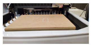
This material sits on top of the machine table loosely until the vacuum table is turned on in the milling process. Your PCB material will sit on top of this material. It is
